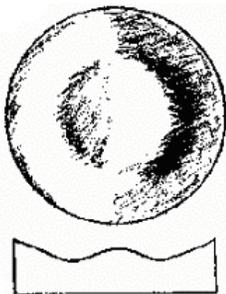
In the first example, we have a central bump, where the centre of the mirror is higher than the surrounding areas. To fix this, we need to go back to polishing to bring the entire surface back to a sphere, making sure we're using 1/3rd Centre over Centre strokes with even pressure. Also, check the pitch lap to ensure that your channels are open and that you have good contact during pressing. An hour of polishing and a short figuring session should correct this issue.
