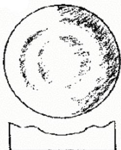
A similar issue that's a little easier to fix is one or more raised ridges on the mirror – again, check your lap and make sure it's in perfect contact, then use a chordal stroke with the tool centred over the radius where the ridge occurs. Do an even number of turns around the mirror for a short while, then check the result when the mirror cools.
